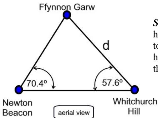
**Step 1:** From each hill, the angle of Ffynnon Garw to the other hill is measured. The horizontal distance from Newton Beacon to Whitchurch Hill is 1840 feet. Use this information to find the horizontal distance,  $d$ , from Ffynnon Garw to Whitchurch Hill to the nearest foot.
